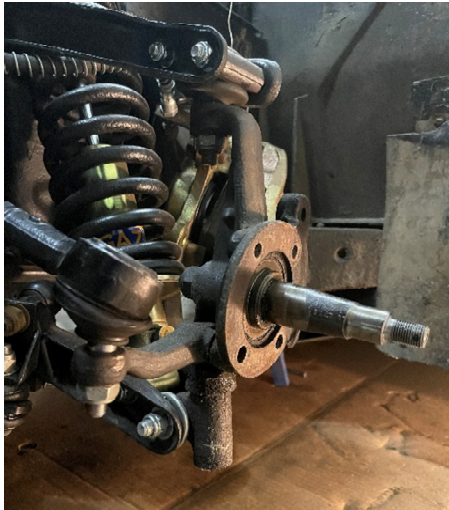
Figure 3 - Rotor & Backplate removed
