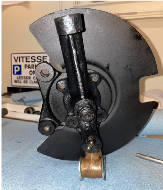
Figure 8 – Assembled vertical link
