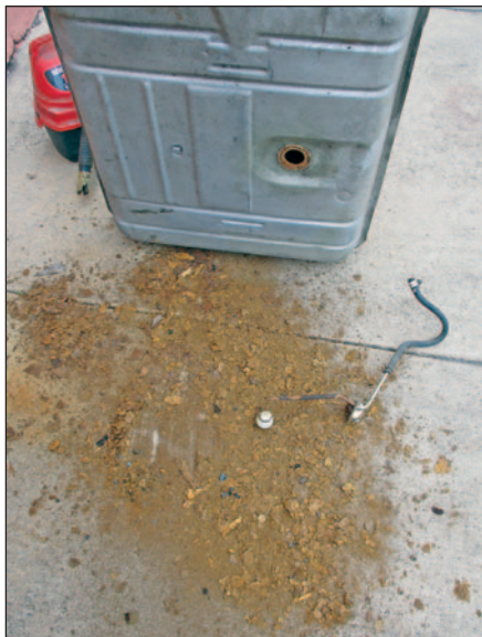
This is what happens when E-10 fuel is allowed to sit in a relined 1956 Buick gas tank for four years. Photo by Pete Phillips
