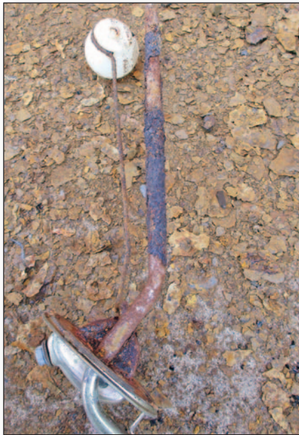
This is what a new sending unit looks like after four years of exposure to ethanol or E-10 fuel. Photo by Pete Phillips
